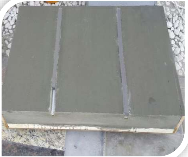
7. Finished Poly Flex, Backing Rod & Bitumastic
